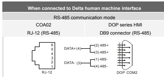
See below communication wirings when COA02 is connected to an equipment through PORT2.
