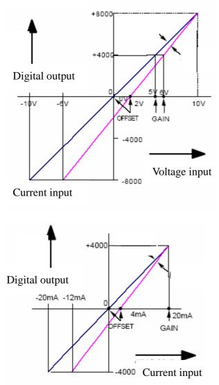
GAIN is the value when digital output equal to 4000 OFFSET is the value when digital output equal to 0 So if set GAIN=5, OFFSET=0 the converting curve is Y=800X, Y is digital output, X is analog input
