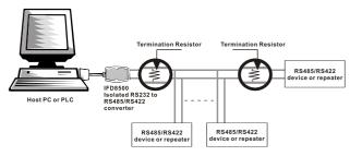
C.If the transmission wire of RS-485 is using AWG#24 twisted pair cable with 1.2km, We recommend you to use 120 Ohm resistor.
